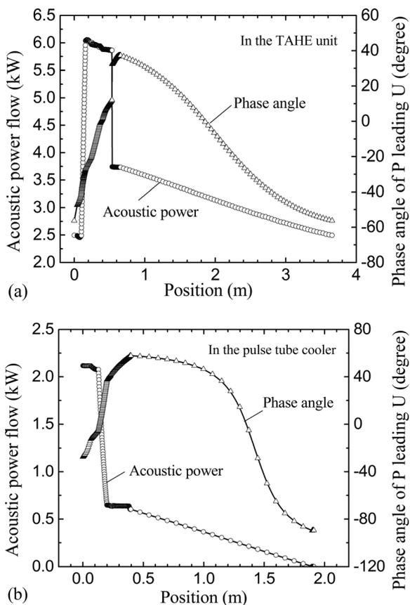
FIG. 2. Calculated results, distributions of the acoustic power flows, and the phase difference between pressure and velocity (a) in the TAHE unit and (b) in the pulse tube cooler; P means the pressure and U means the velocity.
