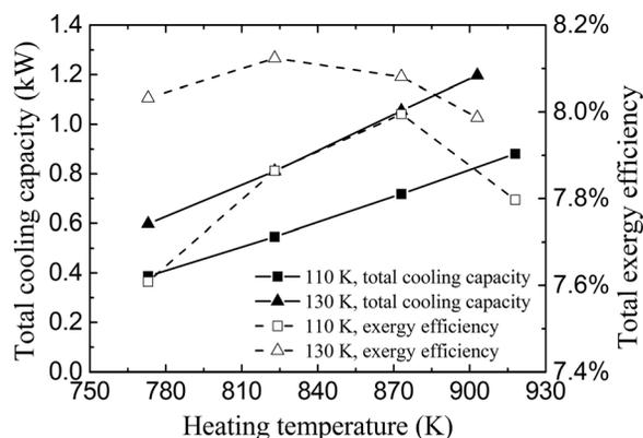
FIG. 3. Experimental results, total cooling capacity at 110 K or 130 K, and the exergy efficiency vs. heating temperature.
