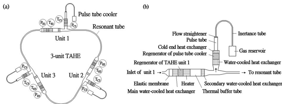
FIG. 1. (a) Overview: the 3-unit heat-driven thermoacoustic cooler. (b) Unit 1 of the system.
