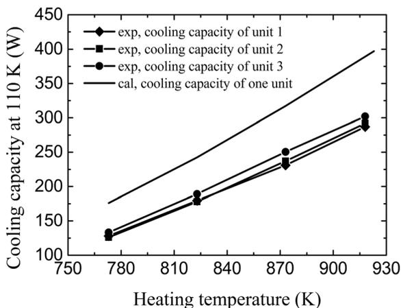
FIG. 4. Experimental and calculated results, cooling capacity of one unit at 110 K.
