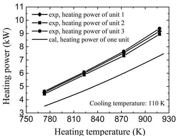
FIG. 5. Experimental and calculated results, heating power of one unit.
